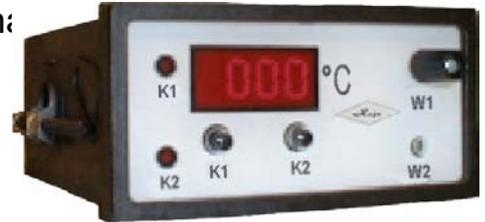
RLCW/48 digital controller are electronical low-cost-devices with 2 switch contacts in spacesaving version. The contact K1 is the control contact, contact K2 for additional functions like cooling, alarm etc. The actual temperature is shown permanently, setpoint is shown by pressing the button. The values are adjusted by a ten-course potentiometer.
